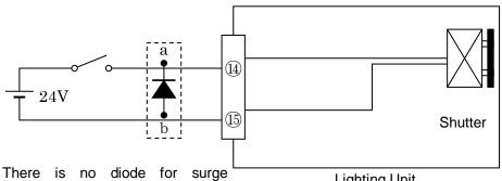
protection connected internally. For connecting an external diode, please refer to the schematic above and to diode specifications below.
